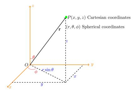
FIG. 1: Cartesian and Spherical Coordinates
